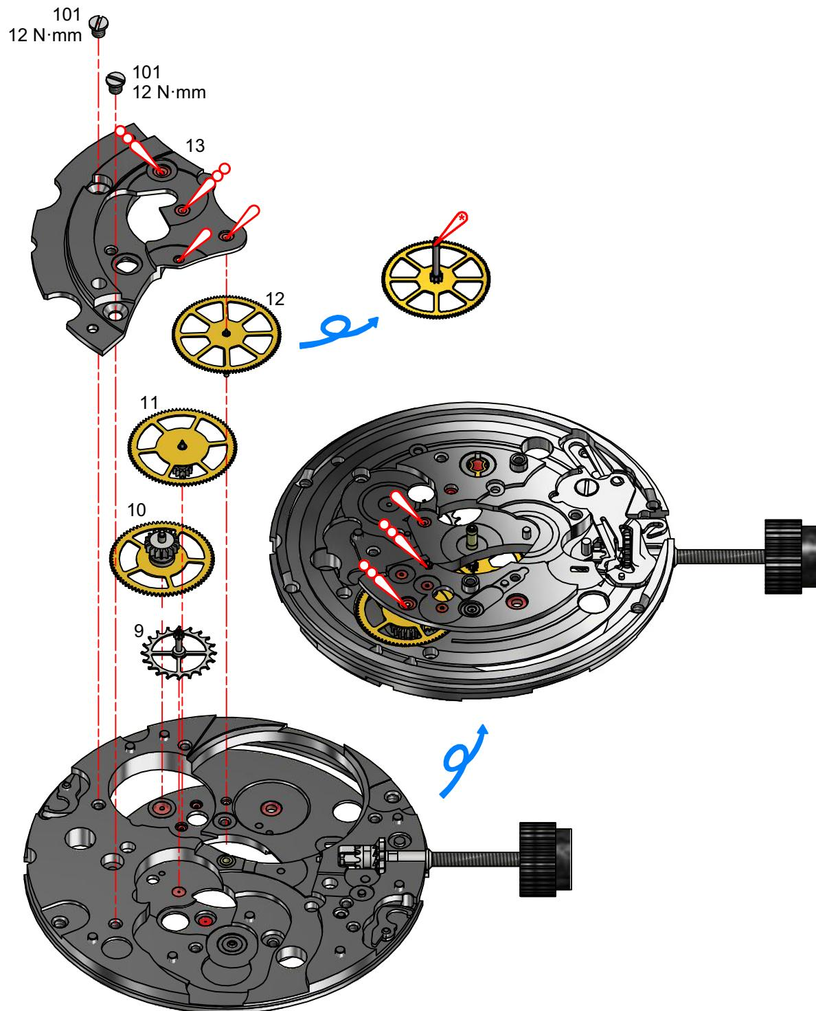
**Montage mouvement – Werkmontage – Assembling of the movement**
