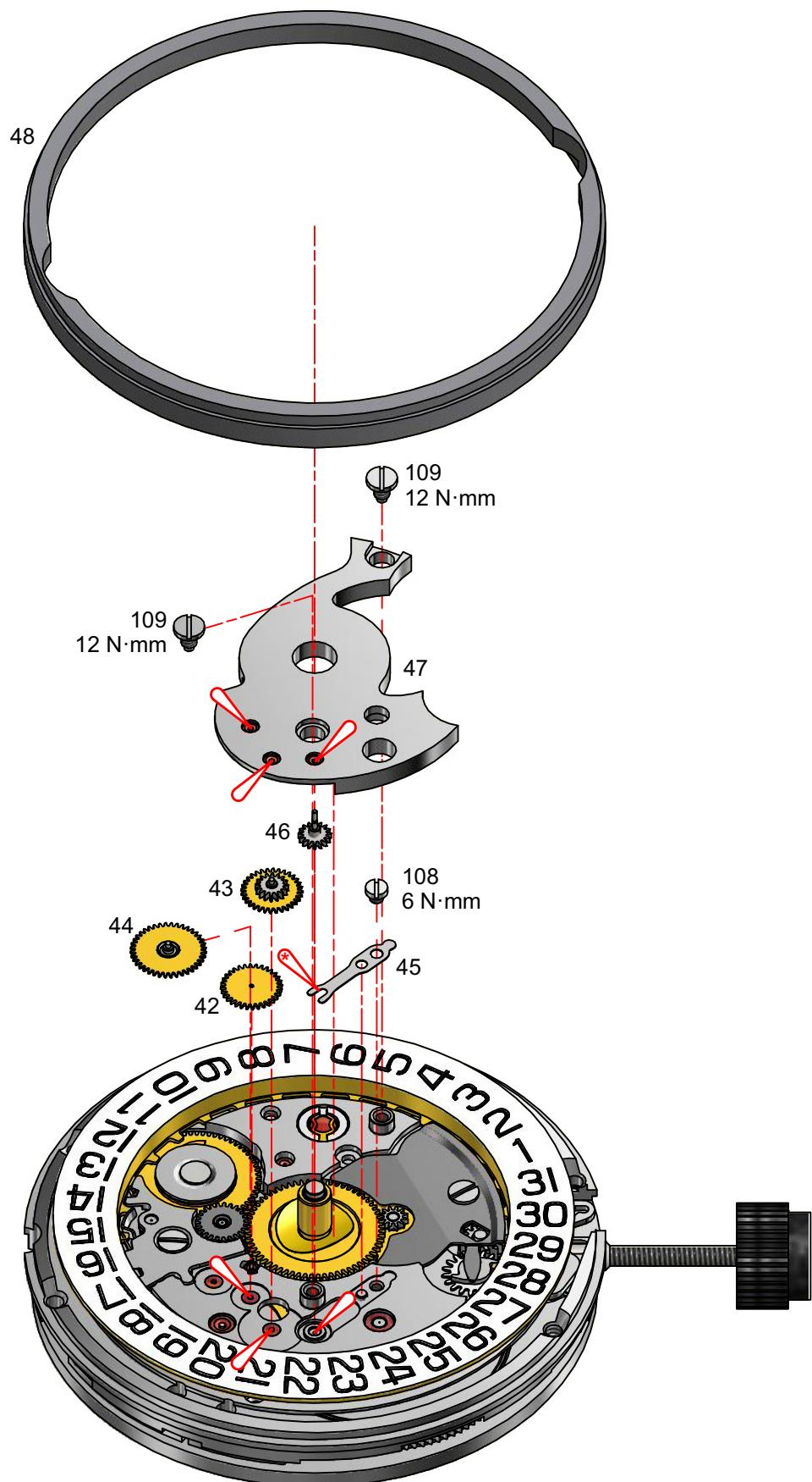
**Montage mouvement – Werkmontage – Assembling of the movement
