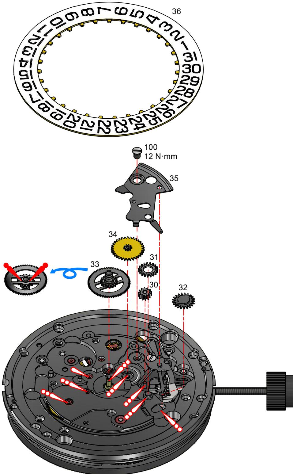
**Montage mouvement – Werkmontage – Assembling of the movement:
